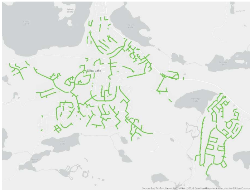
Stormwater Main Criticality Map
